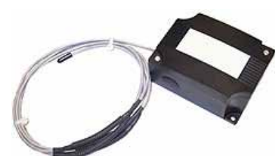
KTT1KP-FD Flex-Duct Sensor – Is made of 20' flexible plenum rated cable which incorporates numerous sensors along the assembly. It acts as a single sensor averaging any temperature change across the sensors.*
