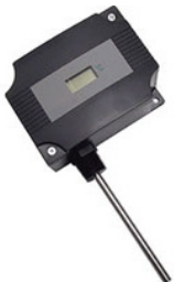
KTT1KP-W Immersion Sensor – Comes with probe and has a 1/2" NPT fitting to be mounted into a brass thermowell (included). Standard 4" length.*
