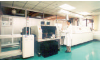
Fully Automatic SMT Line - Screening, Placement & Soldering
