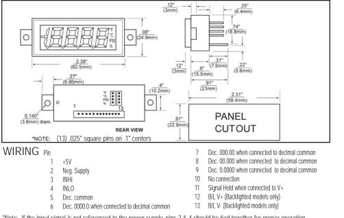
\*Note: If the input signal is not referenced to the power supply, pins 2 & 4 should be tied together for proper operation.
